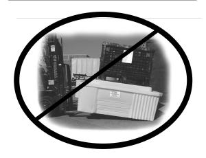
Never move the spill pallet when loaded.
