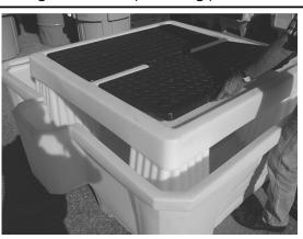
3) Make sure the grates are seated flat on the center pedestal, and the pedestal sits firmly on all four towers.
